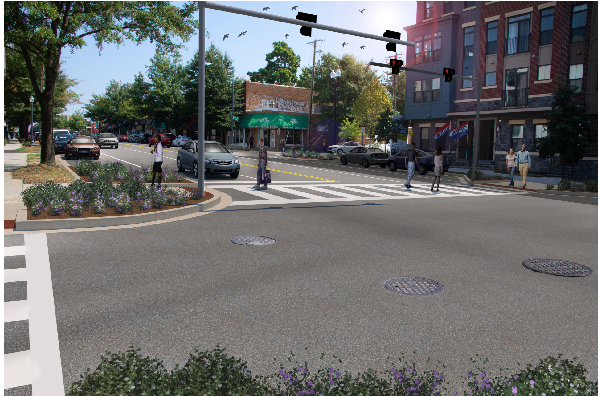
Visualization of Potential Georgia Avenue Roadway Improvements, Including Ladder Crosswalks, Curb Bulb-outs, Planting, and Intersection Signalization
