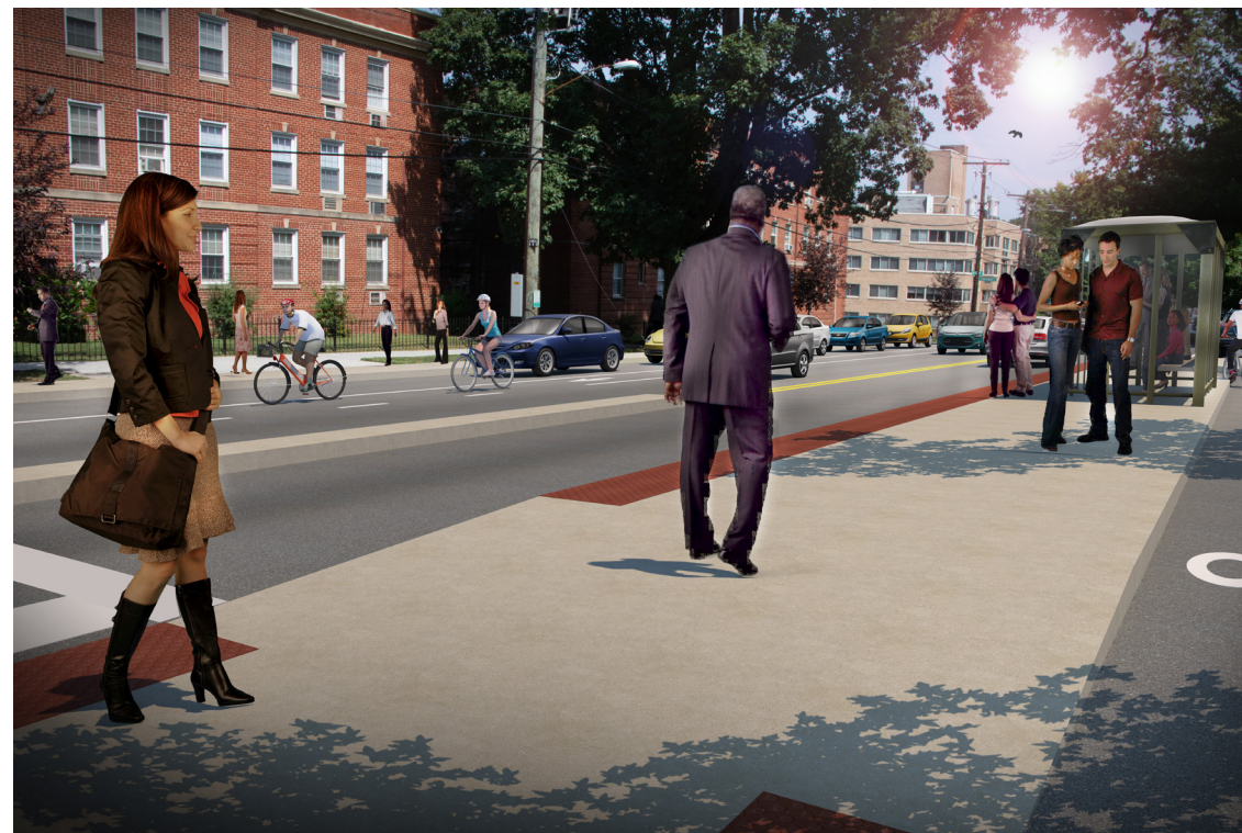
Visualization of Potential Bus Stop Improvements, Showing Floating Bus Stop with Bicycle Facility
